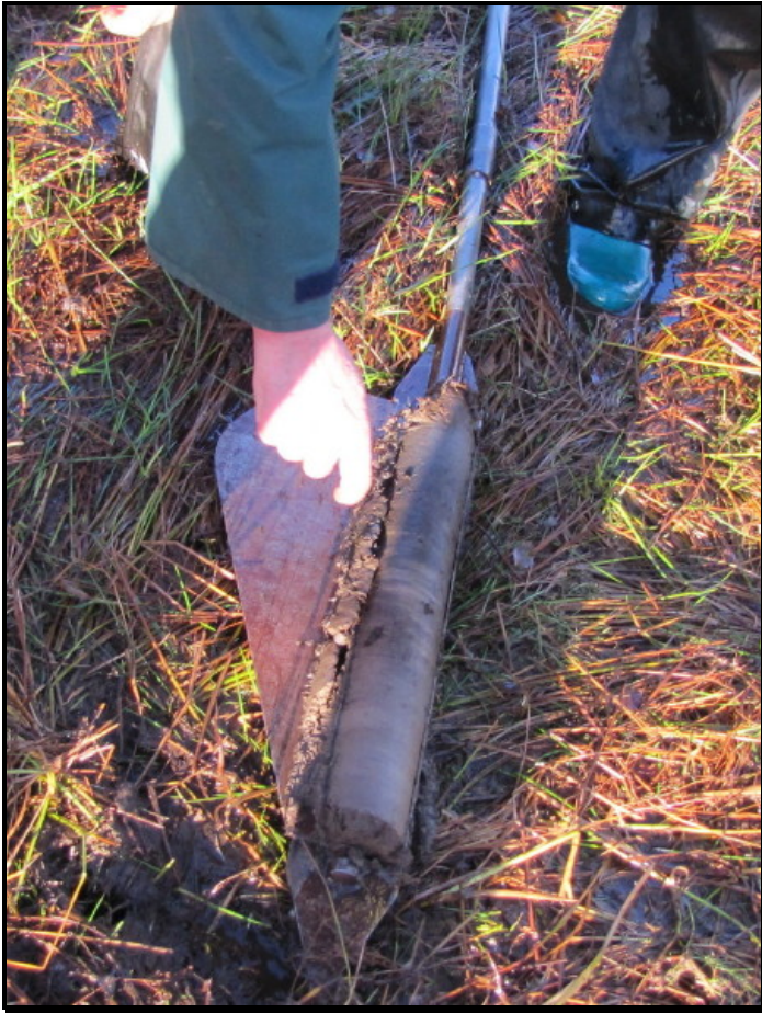
Plate 4: Laminated clays from location 2 in chamber of Russian Corer.
