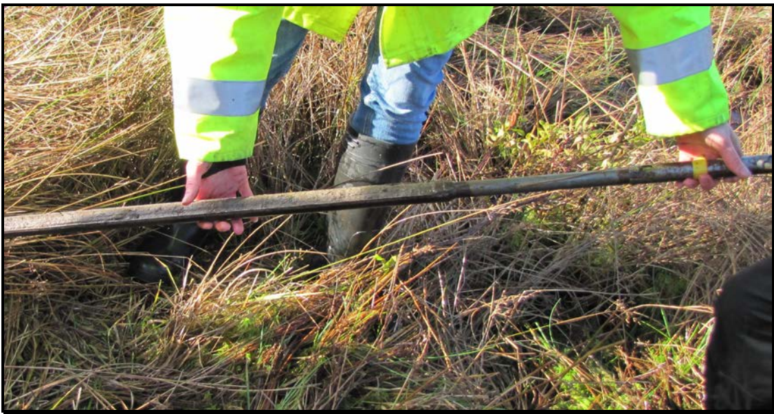
Plate 3: Dutch gouge chamber containing laminated silts and clays extracted from location 1.
