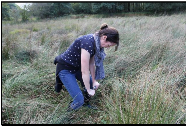
Plate 1: Rapid probing survey using steel peat probes.
