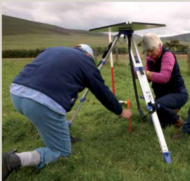
Setting up a plane table and inserting a peg to represent the plane table station. DP098324
